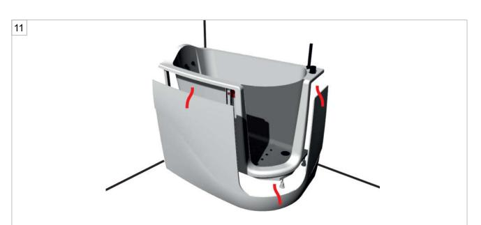
Insert the panel under the tub again, starting from the front side, then under the door and then under the short side.
