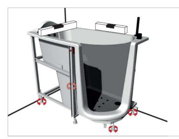
Place the tub in the installation corner and level it perfectly using the feet 1,3,4 and 6.
