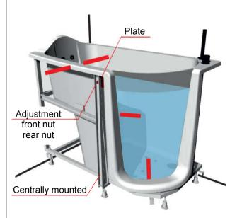
In case of leaks, in the lower part or along the edge near the closing handle, only with a perfect installation as previously described, it will be possible to act on the tub shape by opening or closing the front side. For this aim, on the front frame, there is a column with an adjustment on the head formed by a plate with threaded rod screwed to the tub and two nuts, one placed on the front and one on the back. This system is able to slightly change the closure.
