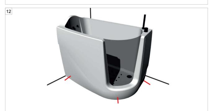
To stop the panel, insert it under the edge of the tub, between the edge itself and the thrust springs. Use the supplied wedges to help you.
